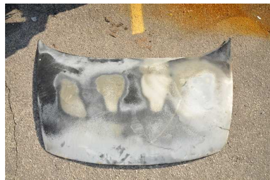
Figure 3: Radial oxide burn patterns on hood.
