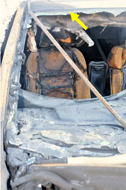
Figure 2: Examination of windshield. Glass is intact at top of windshield and melted at bottom, indicating fire spread from engine compartment.
