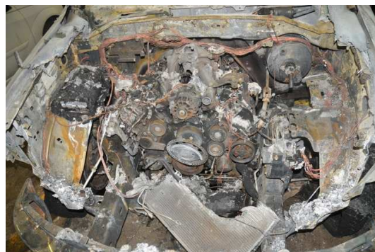
Figure 4: Engine compartment after fire.
